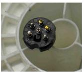
Take the multiconductor cable and approach thge yellow wire from the barrel « 1 ». Make a quick solder of the wire in the barrel to avoid thermal stress on the plastic.
