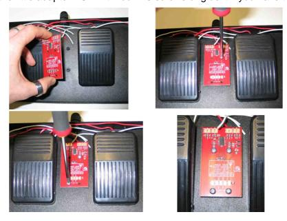
When the PCB is installed, place the top shell beside the bottom one.
