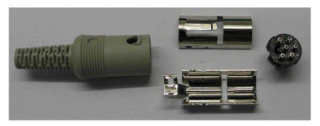
Find something to hold the contacts in place during the wires soldering. The solder spool can do the job.
