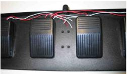
Install the little adapter PCB with four M3 screws or glue it if you have the Eurolite model.
