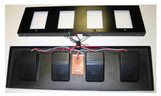
Strip and tin the pedal wires over 3mm.
