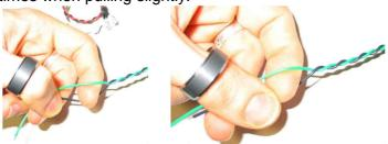
Do the same thing for the green led and the 30cm length black and green wires. Then do the same with the red and white diodes and 20cm length cables. At the end you get 4 assemblies.
