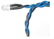
To twist the cables, take the wires between the thumb and forefinger and turn the led several times when pulling slightly.
