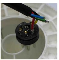
Now for the barrel « 3 » and the white wire, the barrel « 4 » and the blue wire and at last with the barrel « 5 » and the green+black wires.
