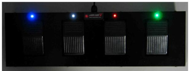
When you press a pedal the led must be turned off to show that the switch operates.
